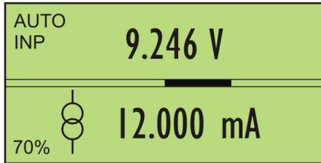
**MULTIMETER** measured input voltage in automatic range.
