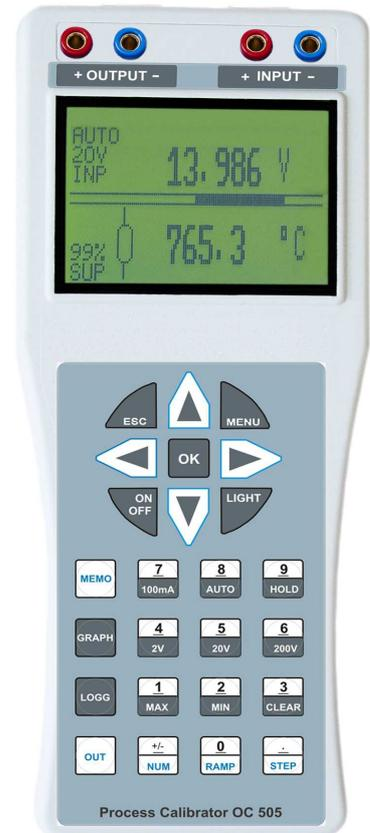
**M505** is a Calibrator-Multimeter for generation of Currents 0-22mA Sink or Source und Voltages to 25VDC. External voltages  $\pm 2V$ ,  $\pm 20V$  and  $\pm 200VDC$  (firm ranges or auto ranging) and Currents to  $\pm 100mA$  can be measured simultaneously and shown at the display.
