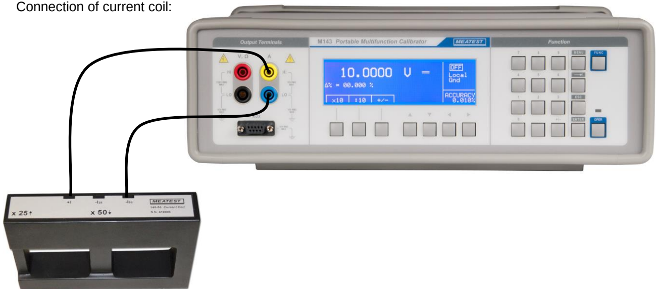
Fig. 25 Current coil connection
